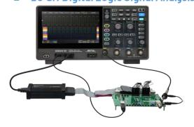
The GPS-2000HD can be used with our 16-channel logic analyser probe option (SLA1016) to add 16 digital channels to the instrument without affecting other test functions, realizing mixed-signal acquisition and analysis, and quickly solving analog-digital mixed-signal design and analysis problems.
